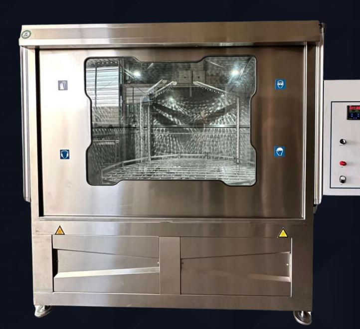
The products are first placed in the rotating basket. It is washed with high pressure hot water and detergent coming from the nozzles in the cabin. Filters inside the machine allow the water in the washing tank to be used longer. Thus, the machine saves water, electricity, time and manpower.
